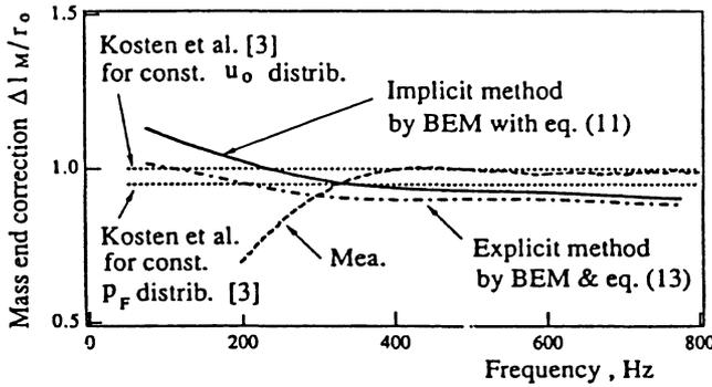
Fig. 3 Comparison of mass end corrections given by the methods.
