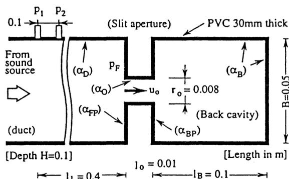
Fig. 1 Slit resonator used in the test.
