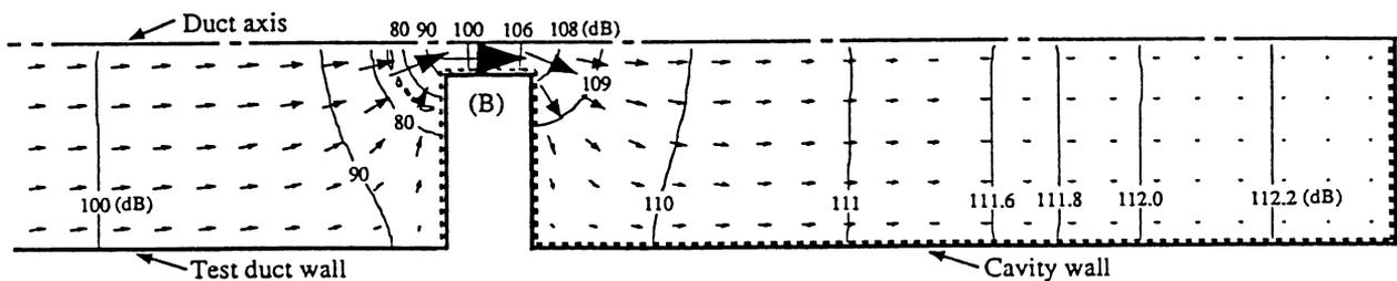
(b) With viscothermal loss ( $R_v/\rho c = 2.0\sqrt{f}\times 10^{-5}$  and  $R_h/\rho c = 0.96\sqrt{f}\times 10^{-5}$ ) on the wall with broken line (----).
