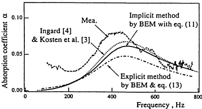
Fig. 5 Comparison of absorption coefficients given by the methods.
