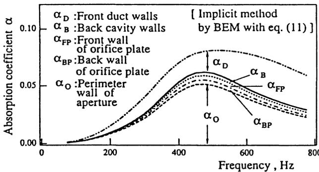
Fig. 4 Each wall contribution to absorption coefficient.
