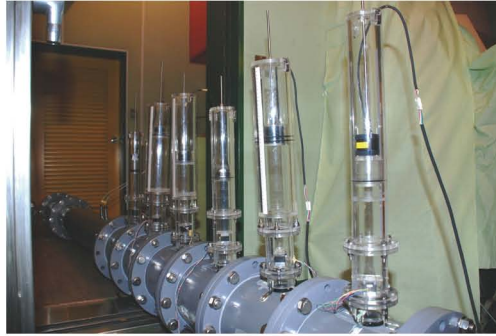
Photo – 3 Prototype tuners attached to a HVAC duct.
