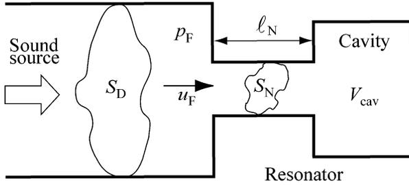
Fig. 1 A Helmholtz resonator at an end of a straight duct
