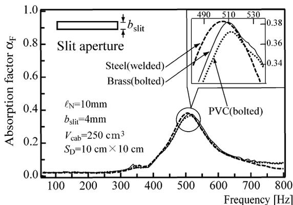
Fig. 2 Dependence of the absorption factor on materials
