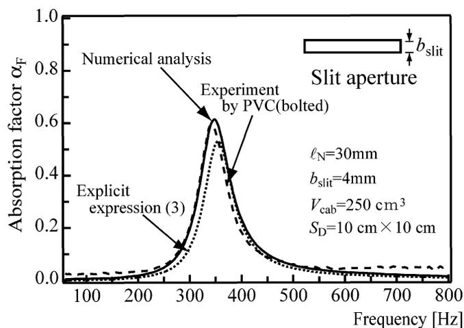
Fig. 4 Effectiveness of the numerical simulation
