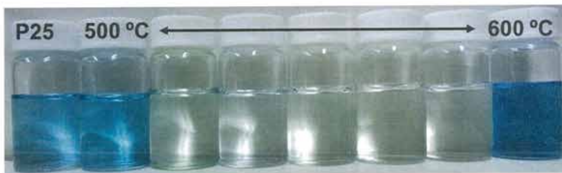
Figure 5-16. Images of supernatant after photodegradation of MB using calcined \mu -PSt-g-PEI@TiO 2 /SiO 2 different calcination temperature for 60 min under visible-light irradiation.
