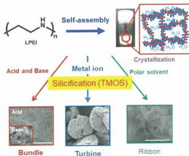
Figure 1-3. Preparation of nanostructured silica by templating PEI aggregates mediated in various conditions.
