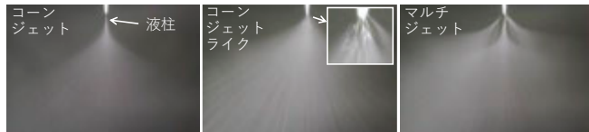
(a) 2.0 ml/h, V_A=7.11 kV (b) 10.0 ml/h, V_A=9.62 kV (c) 10.0 ml/h, V_A=13.2 kV
