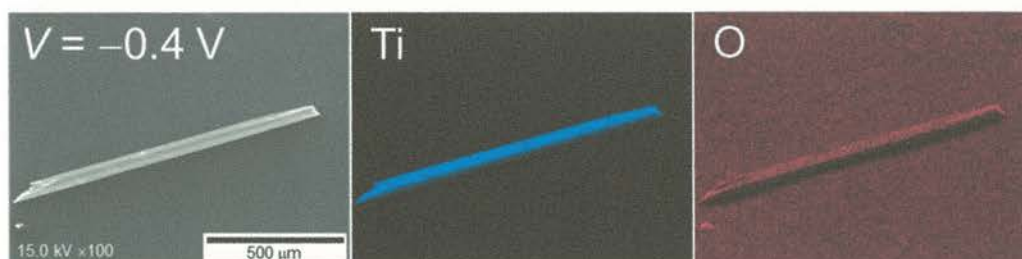
Figure S3.13. EDX mapping images of the \text{Li}_{2+x}\text{Ti}_3\text{O}_7 crystal grown with V = -0.4 V.
