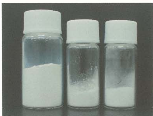
Figure S4.3. Photograph of the (left) \alpha - \text{Li}_2\text{TiO}_3 , (middle) \beta - \text{Li}_2\text{TiO}_3 , and (right) \text{Li}_5\text{Ti}_2\text{O}_6\text{F} powders.
