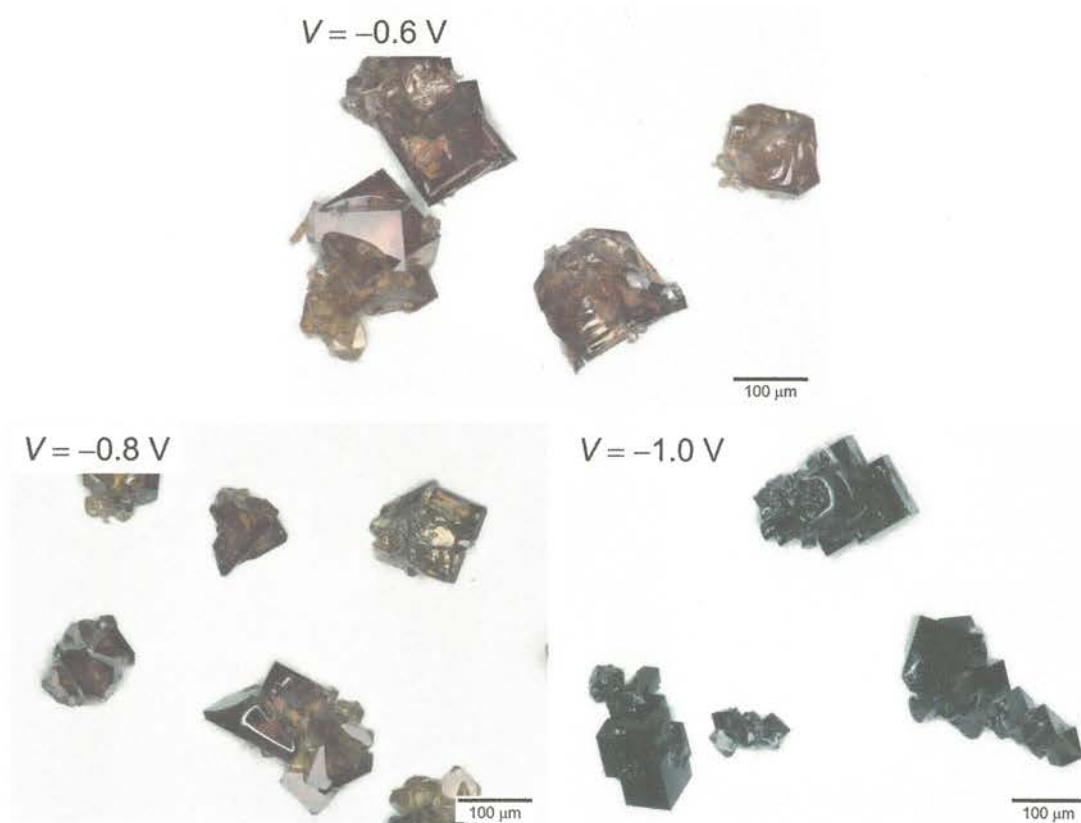
Figure 5.2. Optical micrographs of the resultant crystals grown with V = -0.6 (top), -0.8 (bottom left), and -1.0 V (bottom right).
