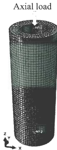
Fig.4.19 Mesh of FE model for CFDST column
