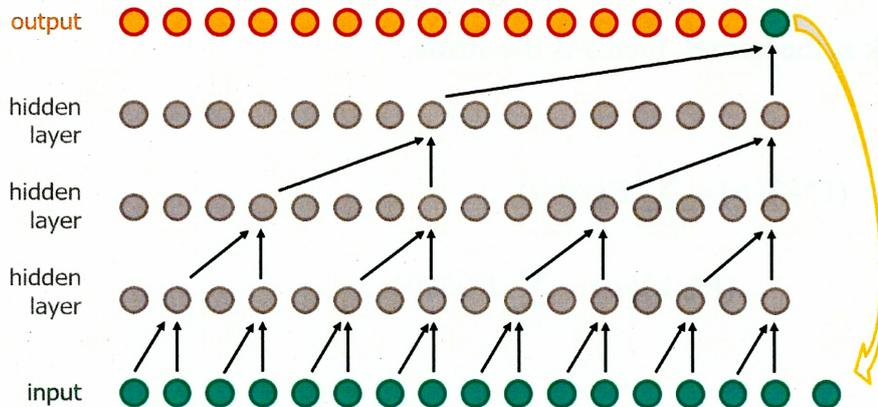
Figure. 5-4 Dilated CNN structure (one-dimensional).
