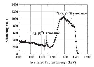
Fig. 4. RBS spectra at the resonance observed for shallowly C-implanted Si (001) substrate with  $4 \times 10^{16}$  cm<sup>-2</sup>.
