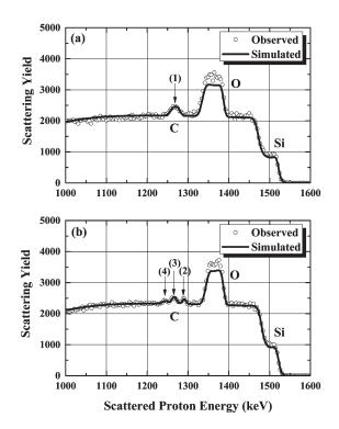
Fig. 5. Resonant RBS spectra observed for the samples as-implanted (a) and post-annealed at 1000  $^\circ\!C$  (b).
