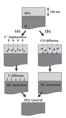
Fig. 1. Formation processes of SiC NCs in  $SiO_2/Si$  samples by C ion implantation (a) and CO thermal diffusion methods (b).
