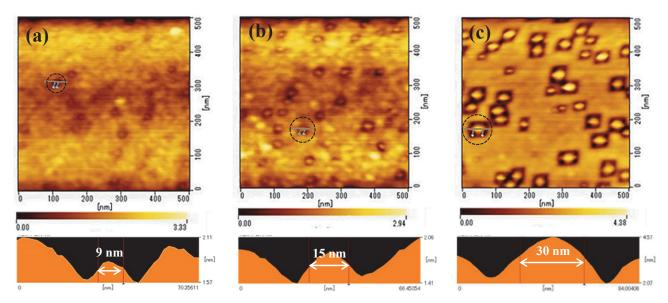
Fig. 7. AFM images and cross-sectional shapes of NC for the samples with different annealing times of 0.5 (a), 1 (b) and 2 h (c).
