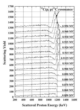
Fig. 3. RBS spectra observed for graphite at various acceleration voltages monitored by GVM.
