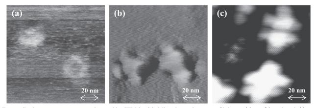
Fig. 9. Surface protrusion images observed by STM for CO diffused samples at 1100°C for 0.5 (a), 1.0 (b), and 2.0 h (c).
