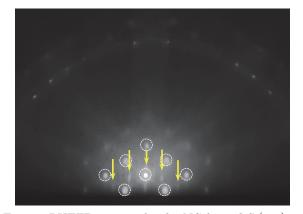
Fig. 8. RHEED pattern for the NC-formed Si(001) surface.
