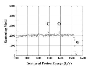
Fig. 6. RBS spectra after eliminating the capped  $SiO_2$  layer entirely.
